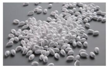
The individual Infinergy<sup>™</sup> beads have a size of from 5 to 10 mm and are supplied with a bulk density of approximately 110 kg/m<sup>3</sup>.
