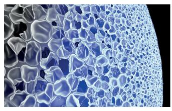
The closed cells inside an Infinergy<sup>™</sup> bead can be seen on the scan taken with the scanning electron microscope.
