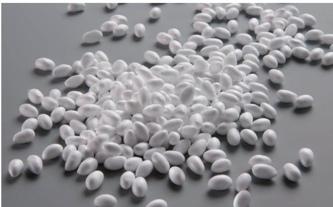
The individual Infinergy™ beads have a size of from 5 to 10 mm and are supplied with a bulk density of approximately 110 kg/m<sup>3</sup>.
